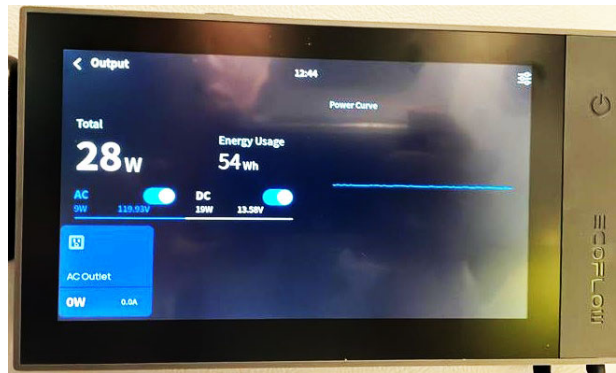
The output screen accesses controls to the output AC and DC. -Typical View
