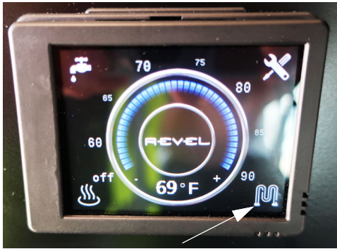
AC Electrical Element Selector (Located near monitor panel) -Typical View
