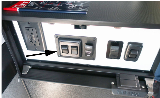
Power Awning Switches and Awning Light Switch (Located near sliding entrance door) -Typical View
