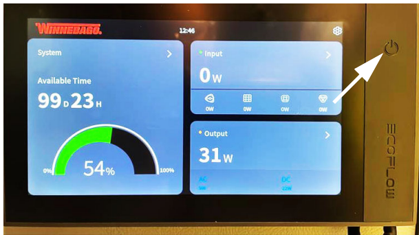
EcoFlow Home Screen- the arrow points to the power button. Press and hold for 3 seconds to turn the power ON. (Press for 0.5 seconds to turn the screen on and off). -Typical View
