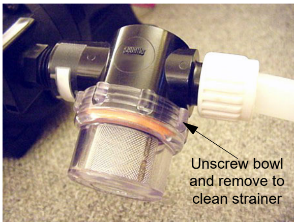
Water Pump Strainer -Typical View
