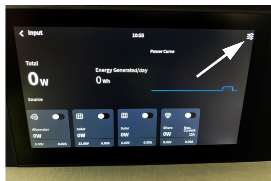
While on the input control panel screen, tap the settings bar icon in the upper right hand corner to open the AC charging current screen. -Typical View
