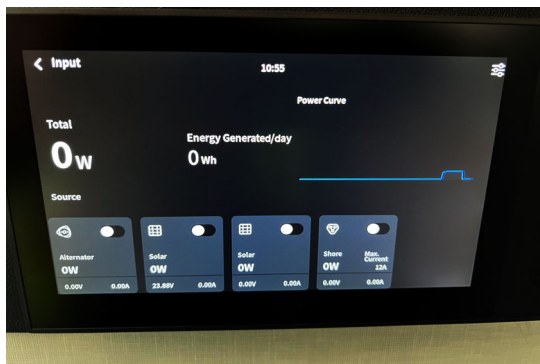
The input screen shows total charging power in Watts, energy generated in watt-hours, and accesses controls of the alternator, Solar, and AC shore power. -Typical View
