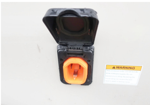
SmartPlug in open position. (Located on the driver's side wall.) -Typical View
