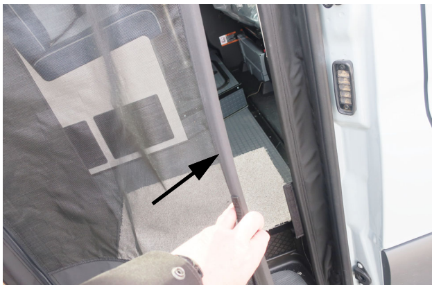
For convenience, the side of the screen has a magnet seal enabling access without unzipping the screen. -Typical View
