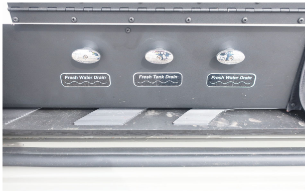
Waterline and Tank Drain Valves (shown in the closed position) (See the “Water System Drain Valve Locations” chart at the end of this section for locations on your model) -Typical View
