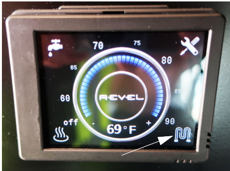
Electrical Element Icon -Typical View
