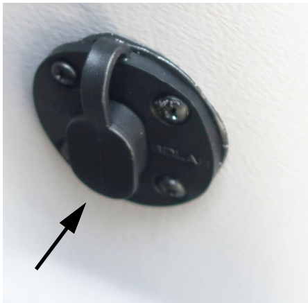
Single Solar Port (Located behind driver's side rear door.) -Typical View
