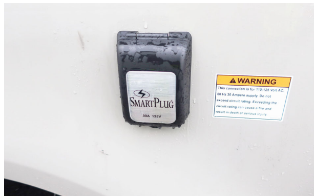
SmartPlug in closed position. (Located on the driver's side wall.) -Typical View
